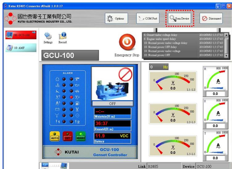
Figure 3-5 Re-Scan for Device
